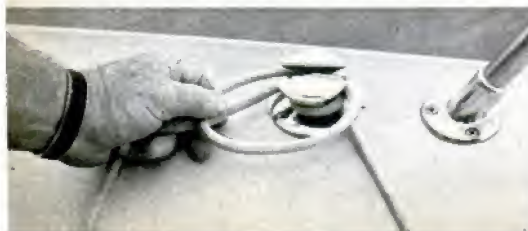
CLOVEN-HOOF and low-silhouette design of Slickcraft cleats makes them less likely to stub bare toes
